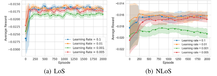
Fig. 3. Convergence of the proposed algorithm under LoS and NLoS assumption.
