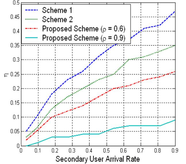
Figure 4. Performance evaluation graph of channel allocation algorithm.
